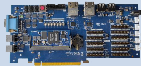
BMC development carrier board with RunBMC installed
